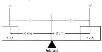
To balance the lever (or scale), how far from the fulcrum must the 12-gram mass be placed?
